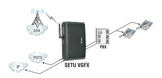
SETU VGFX can be connected to a traditional PBX in two ways. Firstly, the FXS ports of SETU VGFX can be connected to the FXO ports of the PBX. On dialing prefix assigned in the PBX, the user can access these FXS ports to make GSM or VoIP calls. Secondly, the FXS port (SLT port) of the PBX can be connected to FXO port of the SETU VGFX. PBX users can access VoIP and GSM network connected to SETU VGFX by dialing the FXS port number of the PBX.
