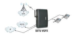
SETU VGFX can be configured in a stand-alone mode by connecting standard telephone instruments to its FXS ports and VoIP-GSM-FXO networks to its respective network ports. Calls over IP are made either through peer-to-peer or using the Proxy Server of a SIP service provider.
