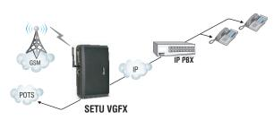
SETU VGFX gets registered to an IP PBX as a client. More than one clients can be registered to a single IP PBX, enabling it to connect GSM and POTS network of various geographical locations.
