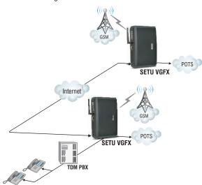
To establish Peer-to-Peer calls, both communicating ends require internet connectivity with fixed IP address. A Peer-to-Peer table needs to be programmed with the IP addresses of the locations and corresponding numeric dialing codes. Using the FXO and GSM ports, SETU VGFX can be connected to local FXO network and GSM network respectively.
